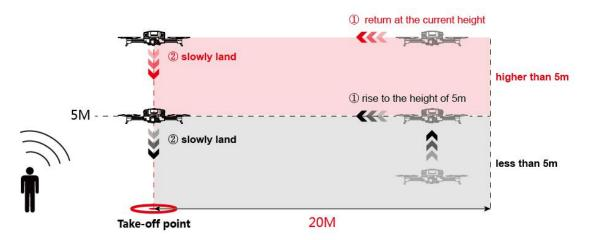
If the aircraft is over 20m away from the return point, the aircraft will rise to the preset height (if the current height is above the set height, the aircraft will fly at the current height), fly directly above the return point, and then slowly land.
