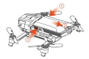
Align the battery with the locking slot of the body, and insert the battery by pushing forwards.
