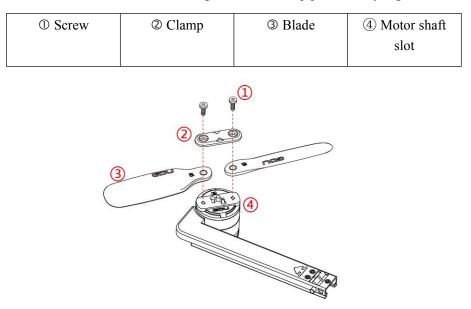
The process of propeller disassembly is as follows. First, remove the screws. Then rotate the clamp of the Type A propeller rightwards or the clamp of Type B propeller leftwards 45 degrees, then remove the clamp. Finally, remove the propeller.
