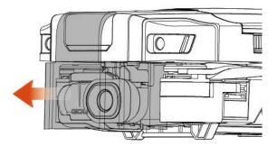
**\*** The cover is used for protecting the equipped gimbal camera. Confirm that the holder cover has been removed before using the aircraft.
